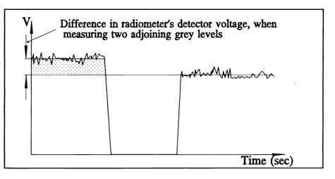
Figure 4: Radiometric measurement of two successive grey levels.
