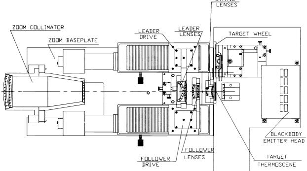
Figure 7: Typical application of a Thermoscene in a dynamic infrared simulation system.
