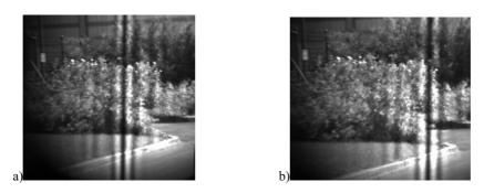
Figure 3: a) FOV frame at the central interferometer position (the central bright fringe is the "zero OPD" fringe); b) the same FOV scene, corresponding to an interferometer off-center angular position: since the interferometer is rotated, the central fringe is not on the central pixel column.
