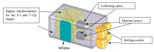
Figure 5: Conceptual view of the dual band IR spectral imager according to the present design. The small optics size and the fact that the collecting optics is made of only two units between the interferometers and the detector arrays, make the instrument especially compact and low cost.
