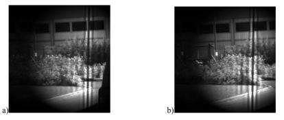
Figure 4: Two CCD acquired images for two optical head angular positions, while the interferometer is stationary in the optical head. The image moves horizontally, while the fringes remain stationary. The optical head rotation is equivalent to the aircraft movement, for the purposes of this explanation.
