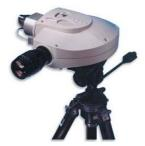
Figure 2: The SpectraCube<sup>TM</sup> based spectral imager (SpectraView), equipped with a telescope lens and mounted on a tripod, for remote measurements of objects in the 0.4 to 1 micron spectral range.
