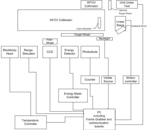
Figure 2: Schematic diagram showing the hardware organization of an EIRT.
